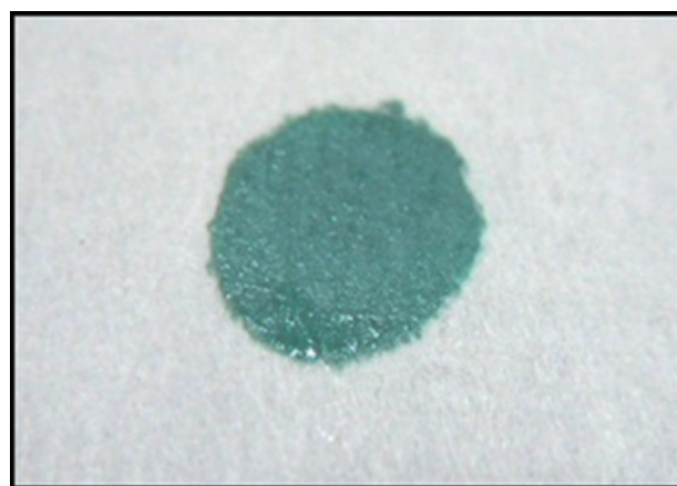
図6 Ni-Cd電池用ポリオレフィン不織布(極液滴下直後) Fig.6 Permeation test of the polyolefin non-woven fabric for Ni-Cd battery
