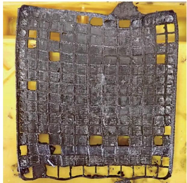
Fig.1 Deformation of the positive plate
