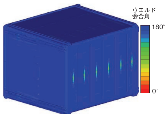
図4 電槽成型時のウエルド会合角解析結果 Fig.4 Calculation result of resin meeting angle during battery container forming
