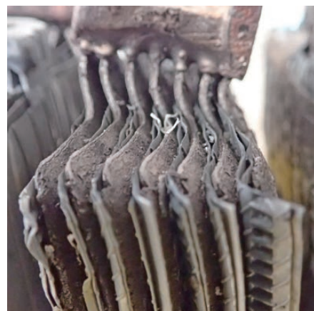
Fig. 2 Out-of-plane deformation of positive plates
