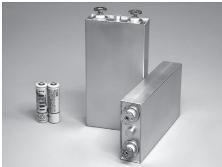
図2 「はやぶさ」用リチウムイオン電池の外観 fig. 2 External View of 13 Ah Class Li-ion cell for HAYABUSA spacecraft
