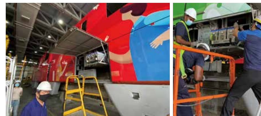
Alkaline storage batteries from Furukawa Battery being installed in Sentosa Express vehicles
